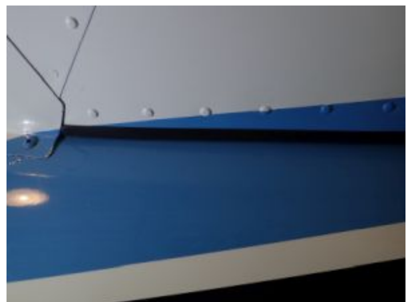
The rubber edge protector is on the rudder, very good extra credit!
