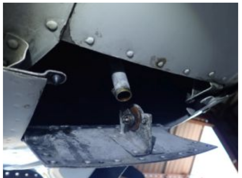
Missing cowl flap bumper.
