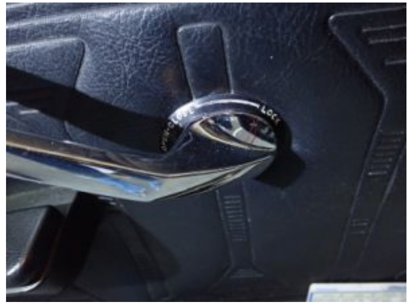
Door handle on one side had a loose bushing/shaft.. may need a rebuilt one in time, or it could be loose mounting screws. We can hope!
