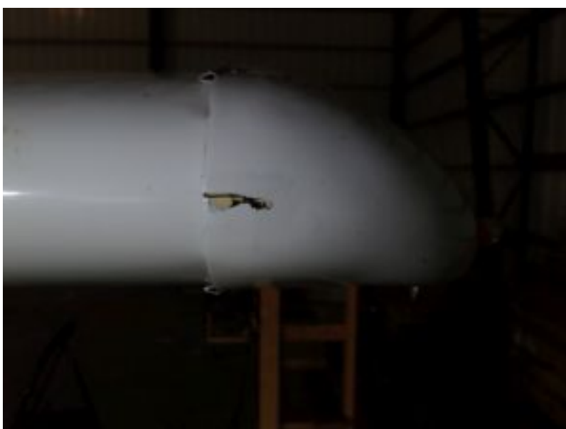
Wing tip crack.
