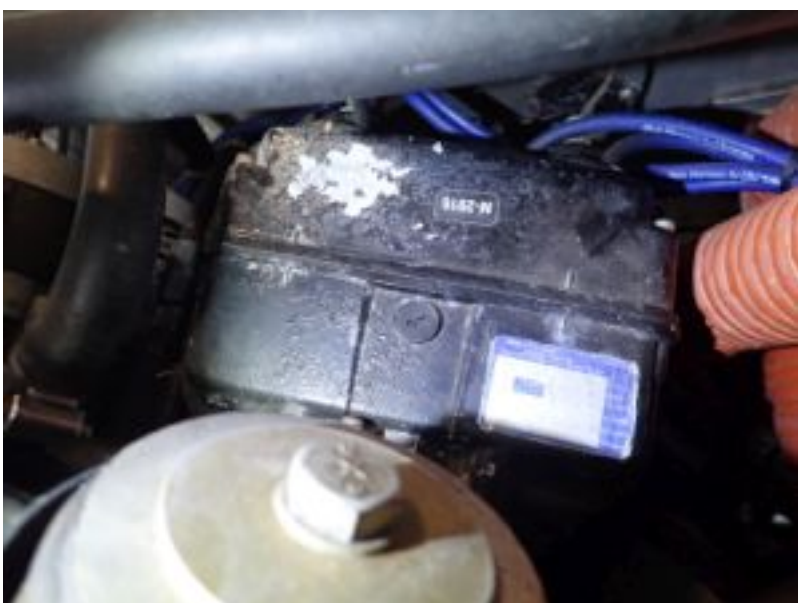
Corrosion on the mag case is very concerning, should be cleaned and painted.
