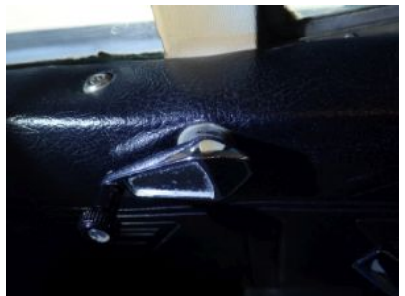
Wing vents needed lubrication
