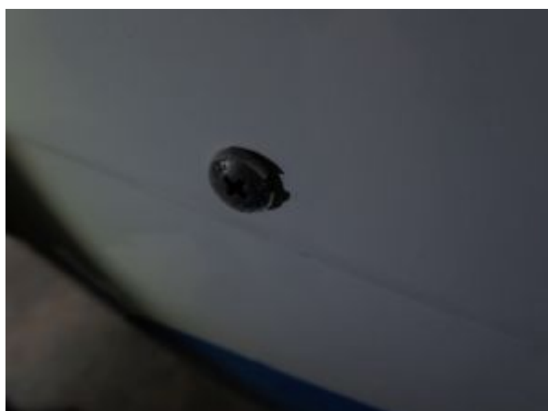
Some cowl screws are 'pulling through' as they are worn out.
