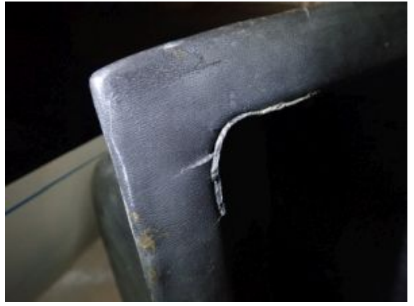
Cracking on baggage bulkhead could be reinforced with Fiberglas.
