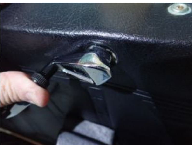
Vent window crank was very worn, ideally find a way to repair or replace it.
