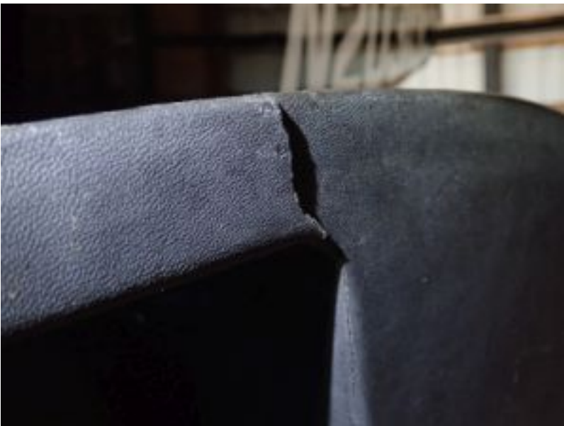
Bulkhead cracks... Fiberglas will make it last, or get a new one.
